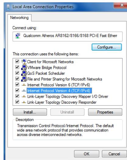
4. Two ways to configure the IP address of PC. **Automatically obtain IP address from DHCP server**
